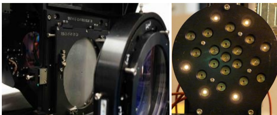
Figure 4: on the left the mask with a 2 mm central hole positioned in the pupil plane, used for the CCD39 centering and conjugation to the pupil plane and for the SEs tip-tilt alignment. On the right the fiber plate containing 23 fibers (1 on-axis) distributed in a 2 arcmin FoV, used during the HWS alignment.
