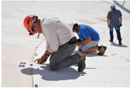
Figure 2. Setting up photogrammetric measurements at the SRT.
