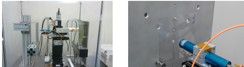
Fig. 5 Setup for the 2D profiles measurements. Left: the CUP setup. Right: the CHRcodile 660 sensor head mounted on the CUP. The glass is supported vertically on three points.
