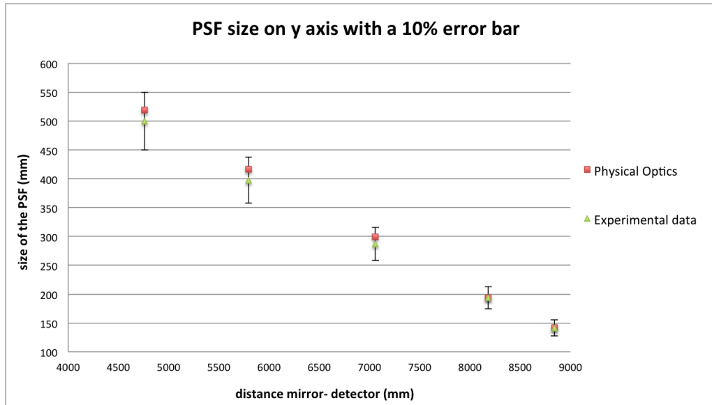
Figure 7. Comparison of the PSF size along y obtained using Physical Optics (red squares) and Experimental images (green triangles) for a mirror oriented at 8.79 deg from the source located at 8430 mm from the center of the mirror with a \pm 10\% error bar on experimental data
