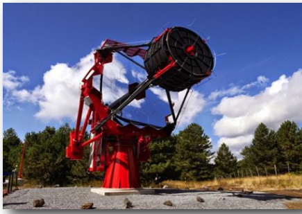
Figure 1 – Left: picture of the ASTRI SST-2M telescope installed at Serra la Nave (Catania, Italy), Right: sketch of the ASTRI Schwarzschild-Couder dual mirror optical design
