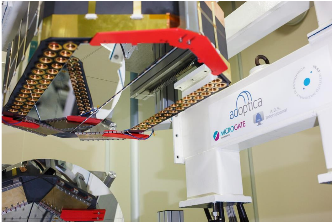
Figure 3. View of the two shells segments mounted on the Demonstration Prototype; some actuators are not covered by the shells, which are undersized because re-used from the previous smaller version of the DP.
