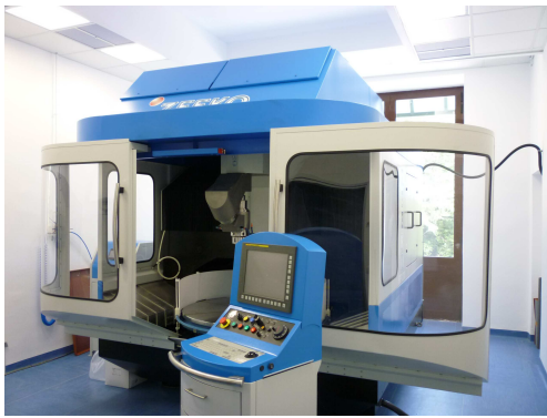
Fig. 1. The IRP1200 series machine in the clean room. The SMU is on the side of the machine, on the left. The SMU feeds the polishing process with recirculating pumped slurry maintained at constant temperature. An integrated density sensor monitors the specific gravity of the slurry.
