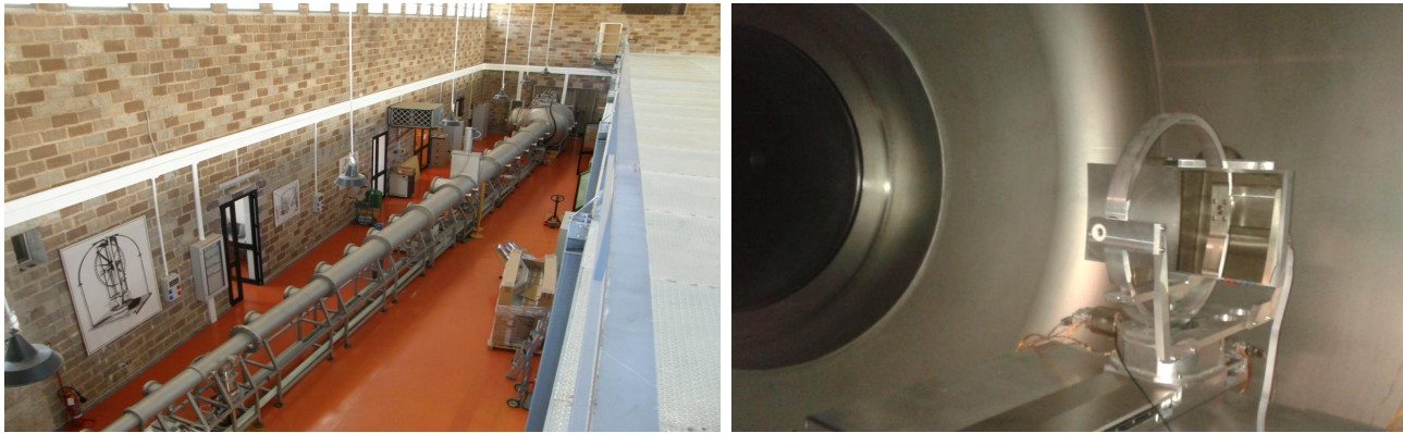
Fig. 5: (left) a view of the XACT X-ray facility at INAF/OAPA. (right) the integrated mirror installed in the manipulation chamber of XACT. Rays impinge from the right side of the image, at an angle of approximately 2.2 deg. The porthole visible on the left side of the picture leads to the microchannel plate detector, at a 4965 mm distance. The module under test is mounted on a translation-rotation manipulator stage, with the optical surface of the mirror at a 210 mm distance from the central axis.
