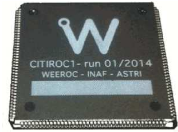
Figure 3: CITIROC chip 4.9 \times 4.6 \text{mm}^2 (courtesy of WEEROC).
