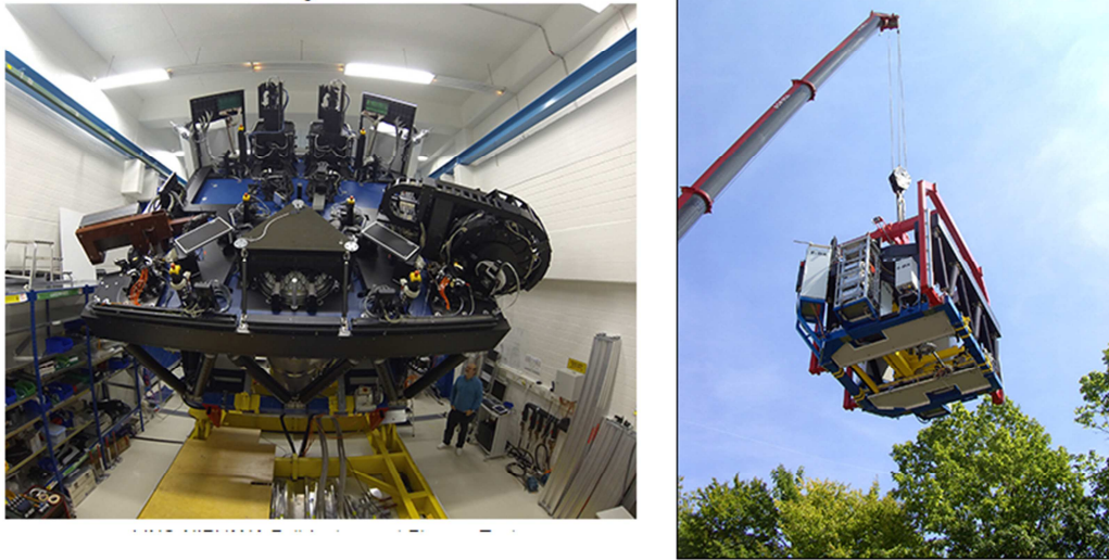
Fig 2: Left: Before PAE, “flexure-test” was performed. Right: “flight-test” before packing
