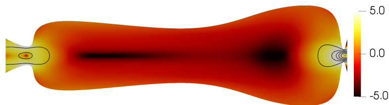
Fig. 4.7 Spatial distribution of the decay rate production in the optimized channel (on a logarithmic scale), \log_{10}(-\sigma_{\Omega}) . Black lines correspond to the oscillating flow velocity magnitude isolines \hat{\mathbf{u}} = \text{const} .
