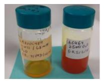
**Figure A.4.16.** Photos of the colour change upon UV irradiation and photoisomerisation. The vial on the left contains 4 wt% C<sub>6</sub>AzoOC<sub>4</sub>E<sub>4</sub> in the native *trans*-state (orange) while the vial on the right shows 2.5 wt% C<sub>6</sub>AzoOC<sub>4</sub>E after UV irradiation (red). It should be noted that in the native *trans*-state, the 2.5 wt% solution is the same orange colour as the 4 wt% solution.
