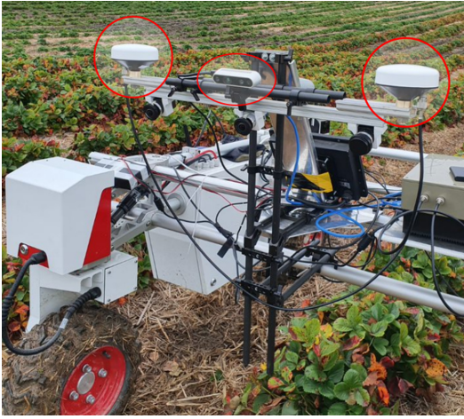
Fig. 4. Our data collection setup showing RealSense camera (for this study we use only RGB images) and dual GNSS antennas mounted on Saga Robotics’ Thorvald platform.
