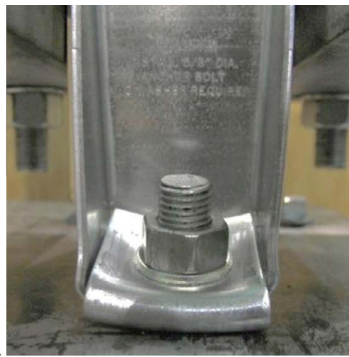
761 Figure 1. Inappropriate failure mechanisms at the connection level: (a) withdrawal of the nails connected to the CLT floor 762 panel; (b) pull-through of the anchoring bolt, (c) tensile failure in the net cross-section of the metal flange, and (d) buckling 763 of the anchoring to the foundations.
