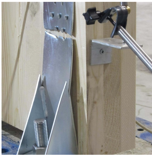
761 Figure 1. Inappropriate failure mechanisms at the connection level: (a) withdrawal of the nails connected to the CLT floor 762 panel; (b) pull-through of the anchoring bolt, (c) tensile failure in the net cross-section of the metal flange, and (d) buckling 763 of the anchoring to the foundations.
