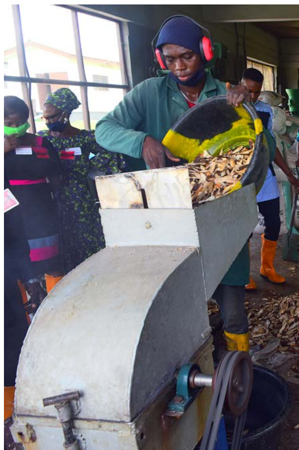
HQCP® production: first step is to grate cassava peels.
