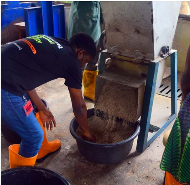
HQCP® production: pulverizing cassava peel cakes into mash.
