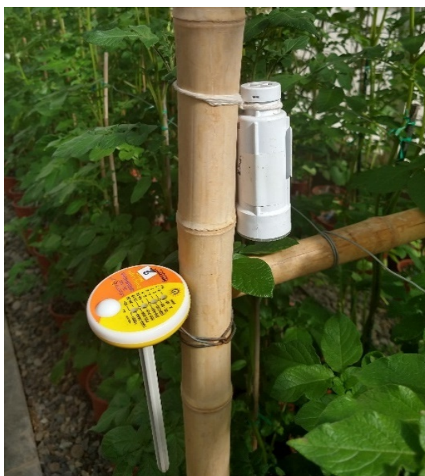
Figure 3. Sensors for DLI measurement (yellow) and for temperature and relative humidity (white).
