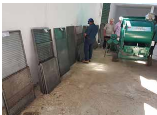
Different sized sieves for various sizes of forage seeds. Photo: Udo Rudiger ICARDA
