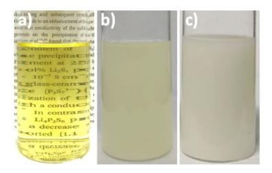
**Figure 1.** Photographs of mixtures of Li<sub>2</sub>S and P<sub>2</sub>S<sub>5</sub> in acetonitrile, in the Li<sub>2</sub>S:P<sub>2</sub>S<sub>5</sub> stoichiometric compositions of **a)** 50:50, **b)** 60:40 and **c)** 70:30 in mol%.
