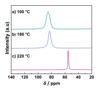
**Figure 4**. <sup>31</sup>P MAS NMR spectra of the 50Li<sub>2</sub>S:50P<sub>2</sub>S<sub>5</sub> sample **a)** after drying at 100 °C, **b)** after drying at 180 °C and **c)** after drying at 180 °C and subsequent heat treatment at 220 °C
