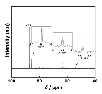
Figure 5.  $^{31}P$  NMR spectrum of the  $50Li_2S:50P_2S_5$  solution.
