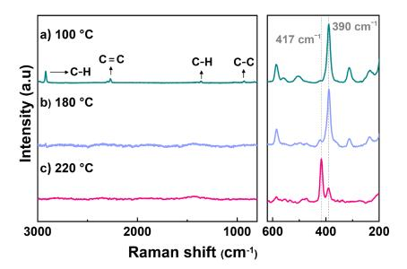
**Figure 3** Raman spectra of the 50Li<sub>2</sub>S:50P<sub>2</sub>S<sub>5</sub> sample **a)** after drying at 100 °C, **b)** after drying at 180 °C and **c)** after drying at 180 °C and subsequent heat treatment at 220 °C.
