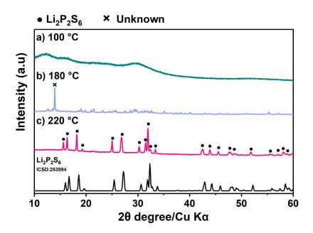
**Figure 2**. XRD patterns of the  $50Li_2S:50P_2S_5$  sample **a)** after drying at  $100 \, ^{\circ}C$ , **b)** after drying at  $180 \, ^{\circ}C$  and **c)** after drying at  $180 \, ^{\circ}C$  and subsequent heat treatment at  $220 \, ^{\circ}C$ . Indexed diffraction pattern of the  $Li_2P_2S_6$  crystal phase (ICSD:253894) is shown for comparison.
