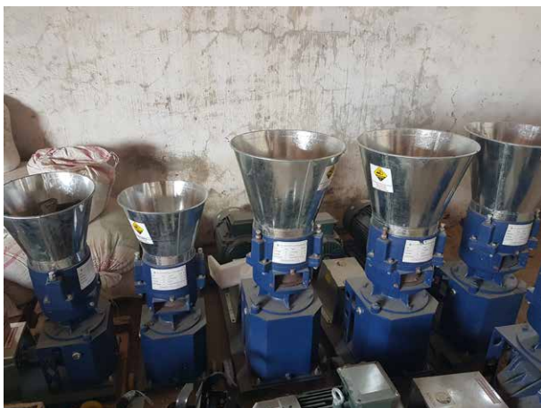
Small pelleting machines. Photo ICARDA/Udo Rudiger
