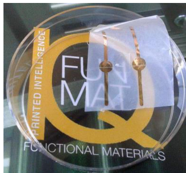
Figure 35 — Left: Typical EIS spectra showing the capacitance (black, f = 10 kHz) and resistivity (blue, f = 1 kHz) of HDF cells attaching and spreading on a 20 nm thick Au electrode film on a nanostructured latex-coated paper. Previously unpublished data. Right: The 20 nm Au electrodes deposited on a layer of nanostructured latex peeled off a paper substrate.
