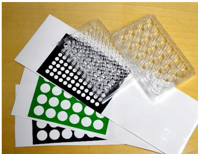
Figure 30 — Images of paper-based screening platforms with geometries similar to those of the commercial plastic 24- and 96-well plates. Green and black wax create the matrix of spherical well areas on the paper-based substrate.
