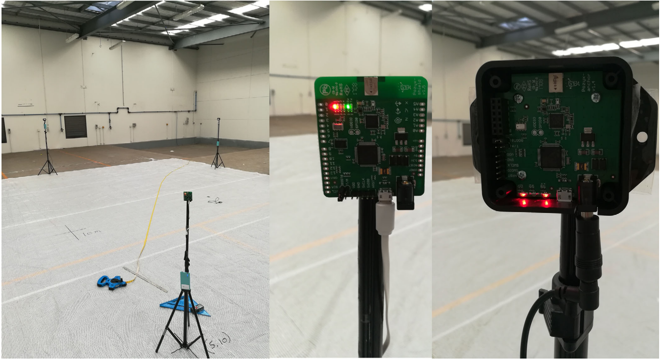
FIGURE 8 Positioning experiment area. (a) Pozyx, anchors and tags used for positioning. (b) Tag (position coordinates need to be calculated). (c) Anchor (known position coordinates)
