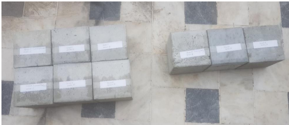
Figure 2. Concrete cube samples (6x6x6 in) of three groups
