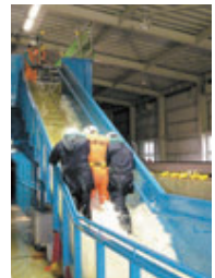
実物大階段模型 (流水階段) Scale model of a staircase (Water flowing staircase)
