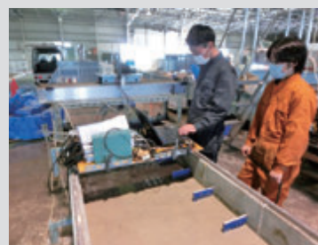
越流による河川堤防の堤体変形実験 Experiment on deformation of river dyke body due to overtopping flow
