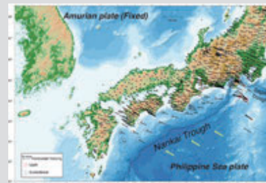
GNSSと海底地殻変動観測で明らかになった西南日本と南海トラフの平均的な地殻変動 Average velocity field in SW Japan and Nankai Trough revealed by GNSS and GPS/A observations
