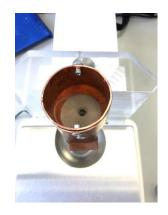
The flowmeter technique for GA powder indicating that powder discharge easily at 1 mm orifice size. The flowmeter technique for HDH powder demonstrating powder creating rat hole at the 1 mm orifice size.
