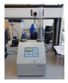
Figure 3. 17 The apparatus of Tapped density equipment
