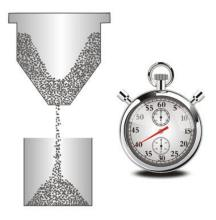
Figure 2. 14 Illustration of powder flowrate measurement (image credit: bettersizeinstruments.com)
