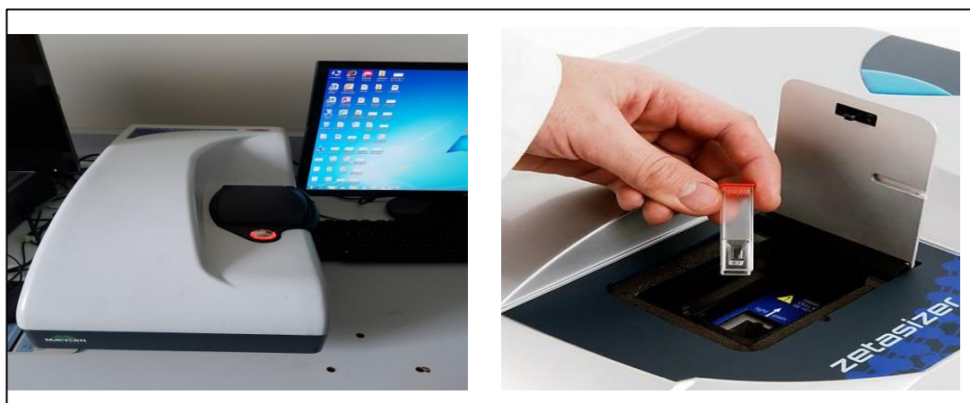
Figure 2.2: Illustrative photos of the Zetasizer Nano ZS-90 during sample loading (Malvern Panalytical Ltd 2018)
