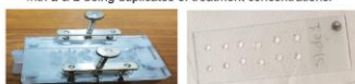
Fig. 2. 12-Gel Comet Assay Unit™ Fig. 3. A slide with 12-mini gels with aluminium base plate holder
