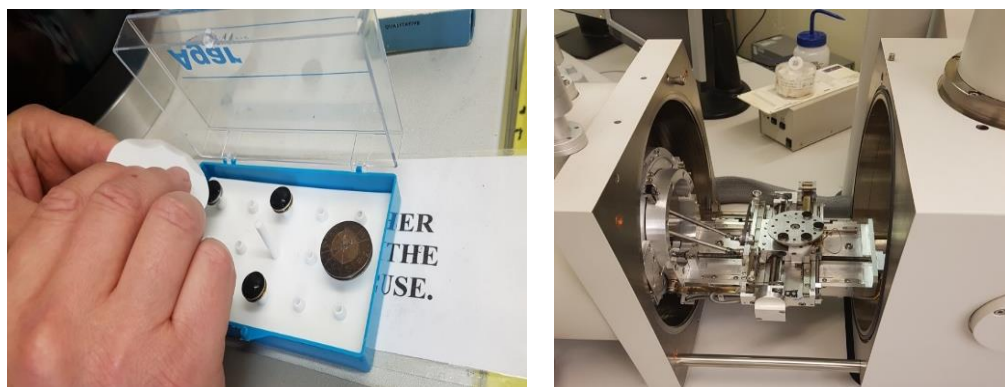
Figure 2.4: Photographic images of the particle preparation on the left and the interior of the SEM during SEM analysis
