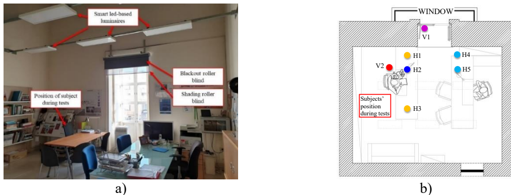
Figure 2. (a) Internal view of the office and (b) office layout with the position of indoor sensors.
