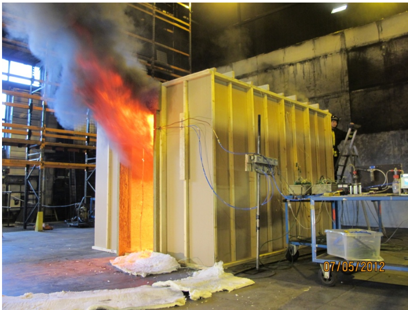
Figure 19. Photo of the room fire test 4. The heat release rate was 1.2 MW.
