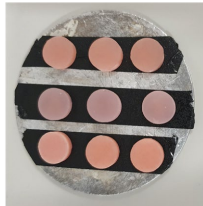
Fig. 2. The cylinder-shaped specimens from groups (CV, CAD, and 3D) used for biological investigations.
