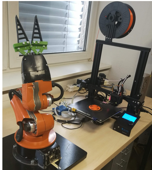
Figure 2: Real world setup with the robot (using a soft gripper) in front of the cartesian FDM printer.
