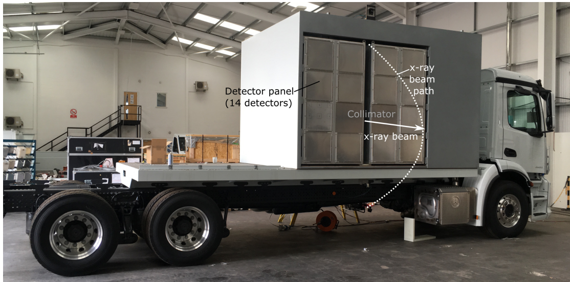
(A) Photograph of a backscatter image system in development showing the detector panel, position of x-ray source collimator and x-ray beam and path. The detector panel contains 14 detectors. The x-ray tube fires x-rays through the vertical gap in the detector panel. The rotating collimator (Fig. B) is used to generate a sweeping pencil beam. The x-ray tube cooling system and the detector acquisition system (Fig. C) are housed behind the detector panel in the container.
