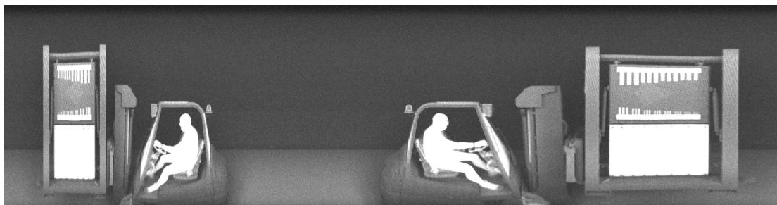
FIGURE 3.4: Backscatter image of a forklift truck carrying a test piece comprised of steel (top) and HDPE (bottom).
