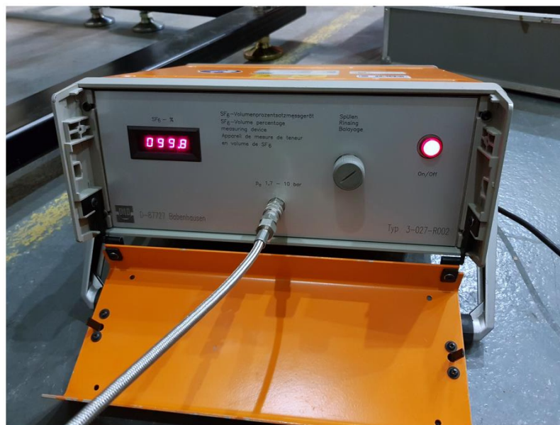
Figure 3-31. DILO SF 6 volume percentage measuring device.
