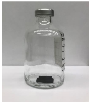
Figure 6-6. EPDM elastomer sample tested for compatibility with C_3F_7CN gas.
