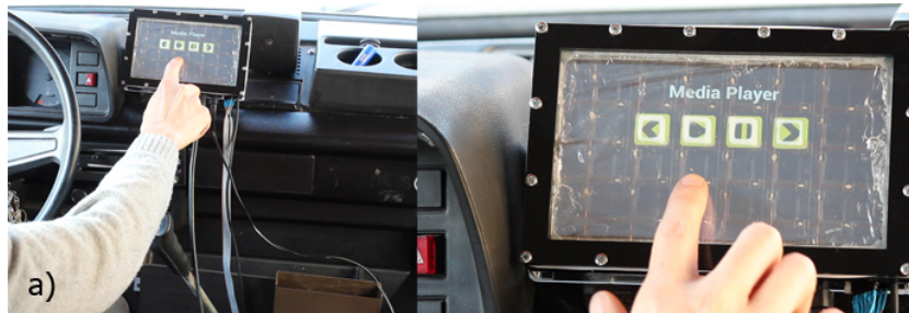
Figure 2.7: Geltouch overlay for touchscreens [15]
