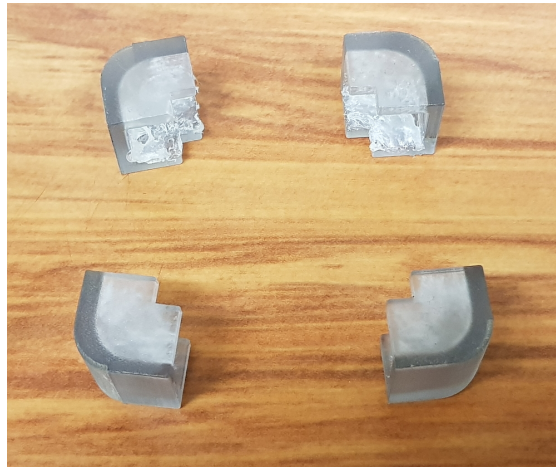
Figure 3.20: Locks used to mount stencils on the touchscreen.
