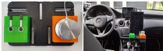
Figure 2.1: Pressure based buttons, physical dial and touchscreen [63]
