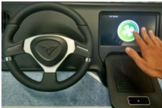
Figure 2.9: Ultrahaptics prototype developed by Georgiou et al. [28]
