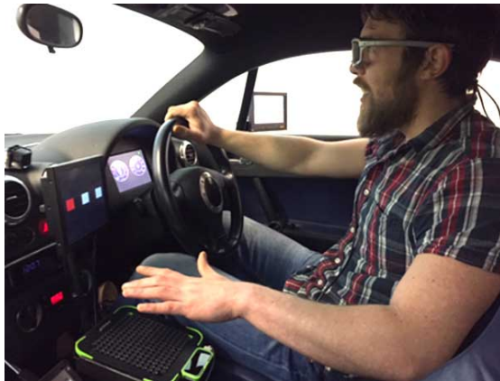
Figure 2.10: Mid-air gestures control with ultrahaptics [33]
