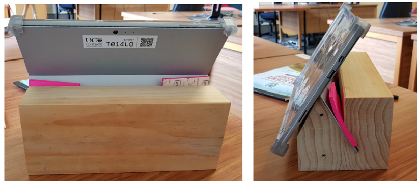
Figure 3.21: Wooden stand used to fix touchscreen on the table.
