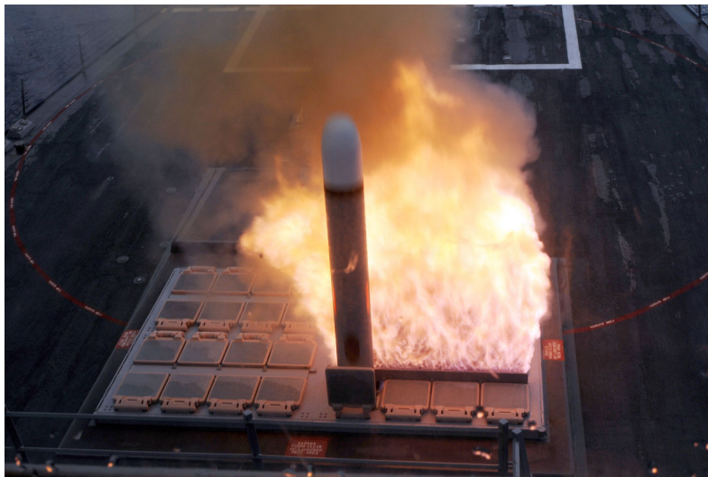
Figure 6. A TLAM being launched from a Mk 41 Launcher. Source: LaGrone (2020).
