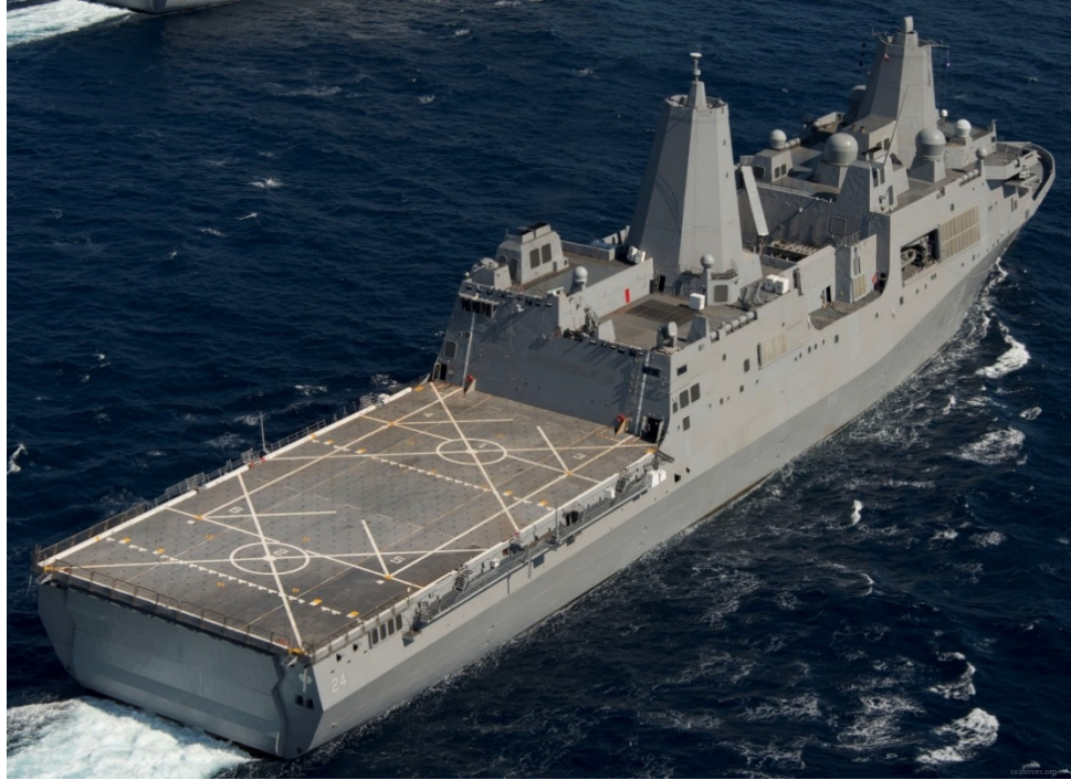
Figure 3. A San Antonio-class LPD highlighting the mission bay adjacent to the flight deck. Source: Seaforce-online Naval Information (n.d.b).
