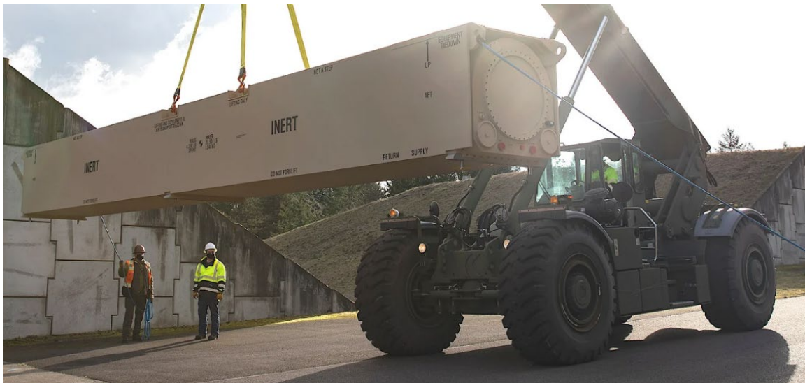
Figure 8. An inert training AUR for the LRHW program. Source: Trevithick (2021).
