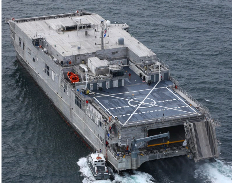
Figure 2. Spearhead-class EPF featuring the flight deck and extensible boom crane. Source: Vavasseur (2020).
