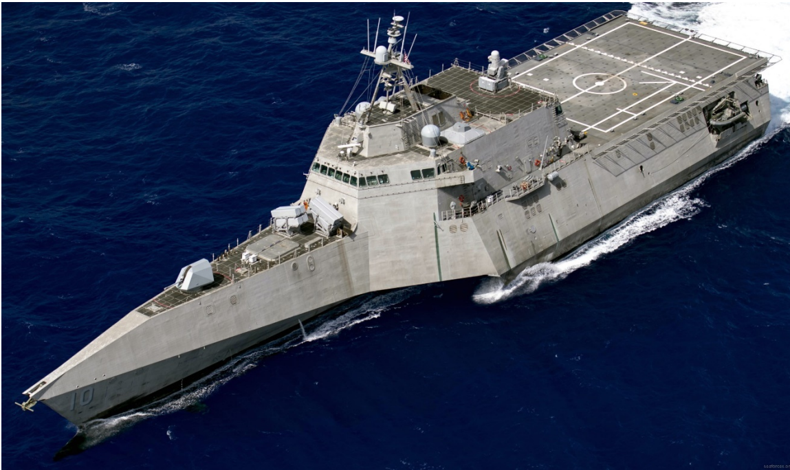
Figure 5. Independence-class LCS highlighting the flight deck and bow missile launchers. Source: Seaforce-online Naval Information (n.d.a).
