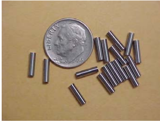
Figure 3.20 NiTiNb plugs (Wu and Schetky, 2000).
