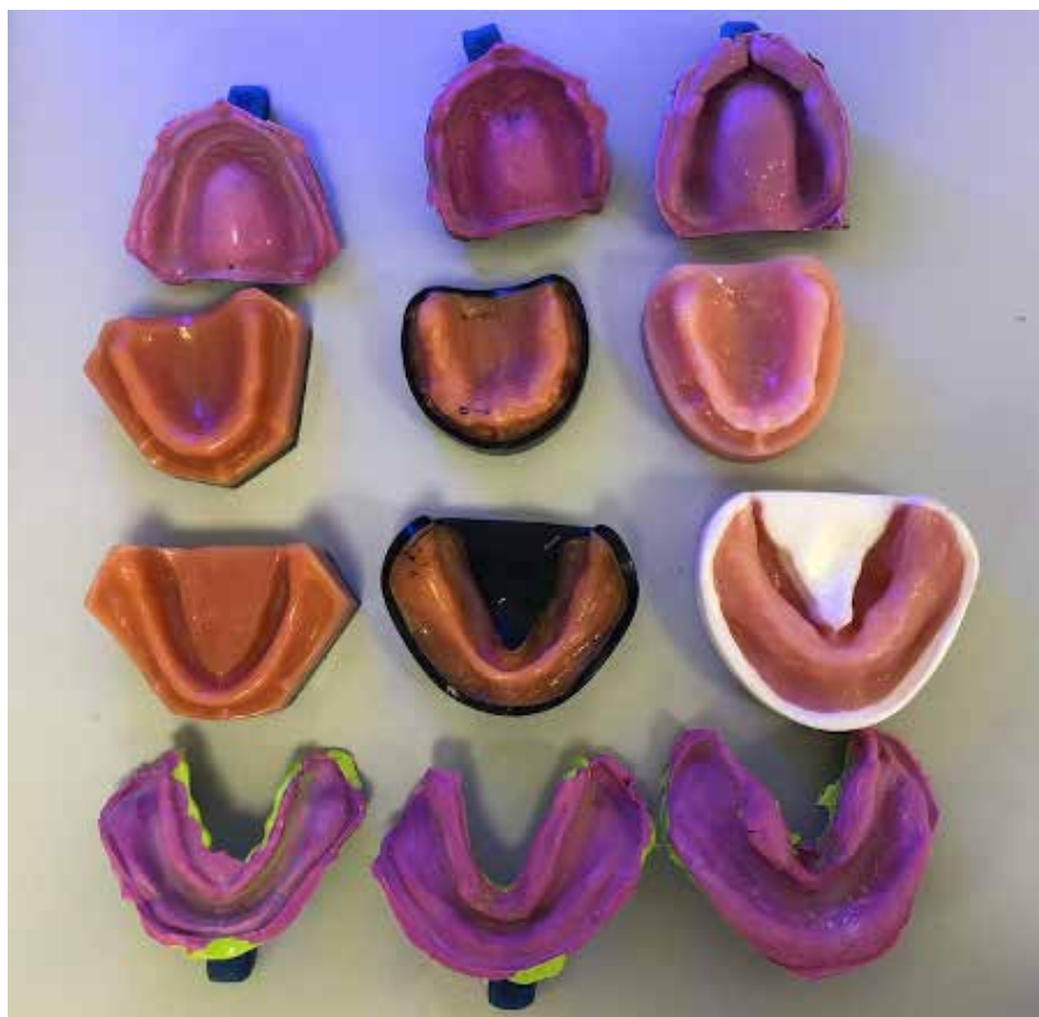
FIG. 1 Three different sets of edentulous acrylic reference models with their corresponding silicone impressions.
