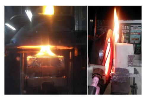
Figure 4. PCM plasterboard burning in the cone calorimeter for the two orientations. Note that in the horizontal orientation the insulation has been removed to show the aluminium block and foil for illustrative purposes only.
