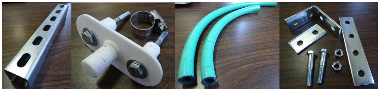
Figure 8: Supplies for Test Rig (l to r): Unistrut C-channel, Boundary Conditions, Hoses, Attachment Hardware
