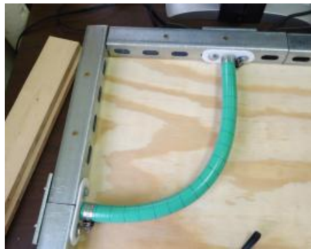
Figure 10: Test Rig with Hose Attached (Shape #6)
