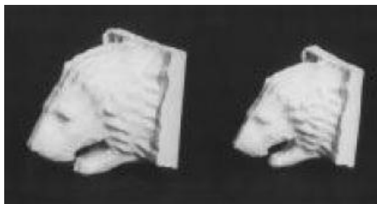
Figure 1.12: Difference of ceramic green and sintered alumina parts made from an organic resin with SL [49]
