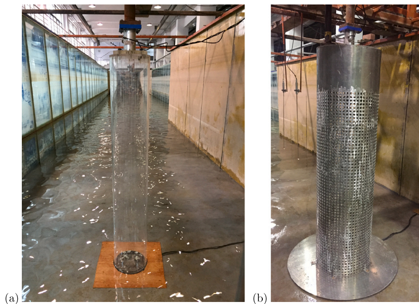
Fig. 2. Photos of fixed cylinder models in the empty tank. (a) Solid cylinder OD 250 mm. (b) Porous cylinder with OD 500 mm and porosity \tau = 0.3 .
