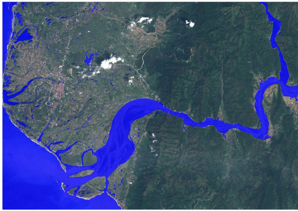
Figure 1. An example of a data product from the Copernicus EMS catalogue (activation EMSR312), in this case a map showing flood extent over the city of Vigan in the North West of Luzon island in the Philippines in September 2018. A blue water mask (here generated using an automatic method from a RADARSAT-2 image) is overlaid on top of a Sentinel-2 image, showing the extent of flooding. Sentinel 2 imagery and Copernicus EMS mapping products are provided as public domain. Base image and reference labels mask are included in the WorldFloods database and code for plotting this images may be found in our repository 6 .
