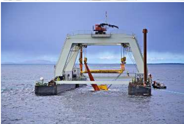
Fig. 10. a. Point-pivoted buoy CAD model with integrated EMG; b. WEC floater following fabrication; and c. gantry barge to be used for deployment.
