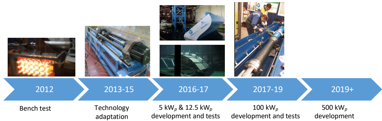
Fig. 3. Major technology steps on the development pathway of the EMG PTO.
