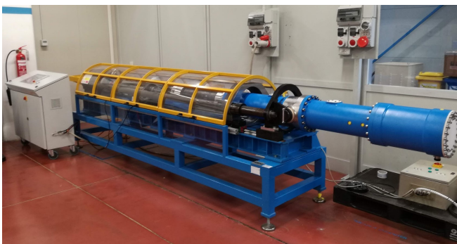
Fig. 4. Factory Acceptance Testing of the 100 kW p EMG
