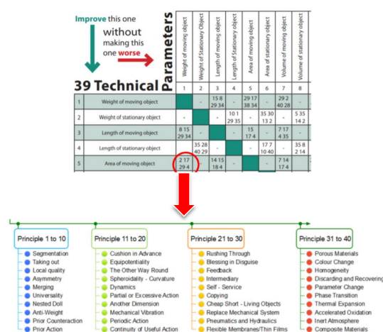
Figure 3. Example of a subset of the TRIZ 39 \times 39 contradiction matrix ( top ) linking to the 40 inventive principles ( bottom ) [30,32]. These are designed to be generic to multiple industries and applications, thus do not specify units.
