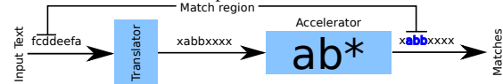
Fig. 2. A stateless translator converting cd* to ab* . x is an arbitrarily selected character to avoid false-positives.
