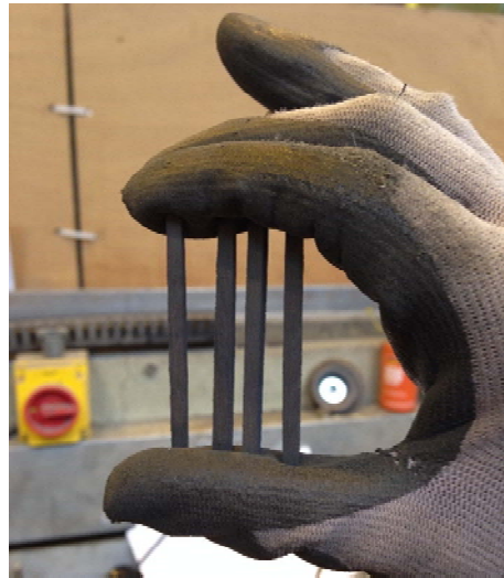
Figure 4. Specimens for DMA tests in three-point bending configuration
