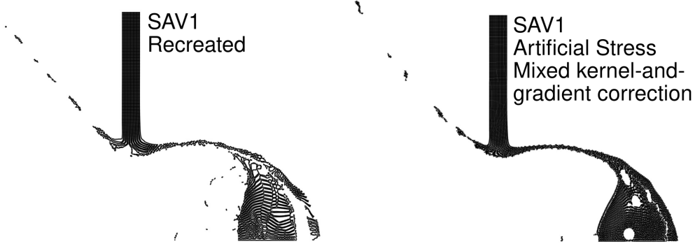
Figure 10: Particle positions of the high-velocity impact problem 8 \mu\text{s} after impact. The results are for the recreated SAV1 scheme from Mehra and Chaturvedi [34] and SAV1 combined with artificial stress and the adapted mixed kernel-and-gradient correction.
