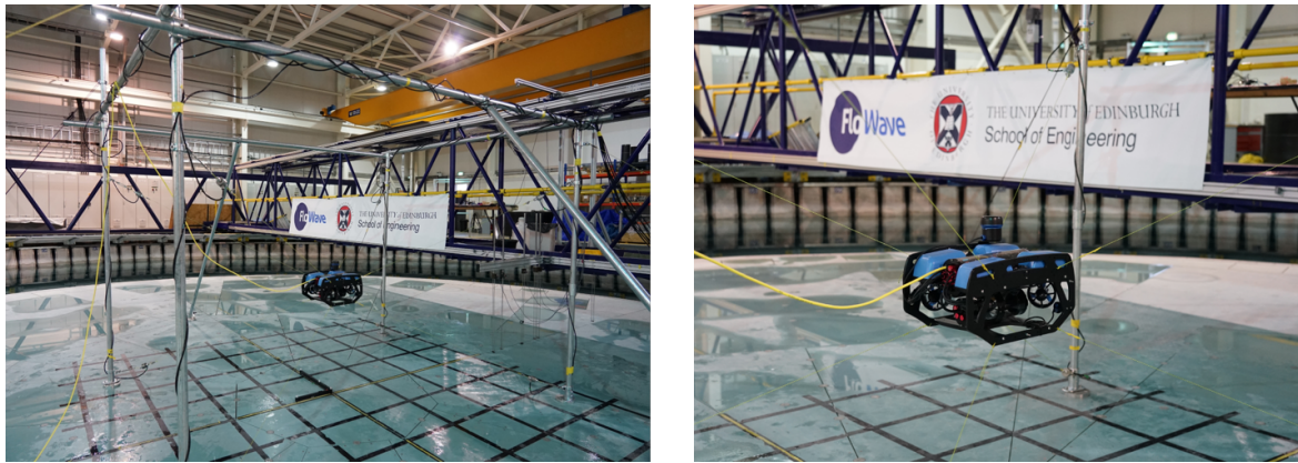
Figure 7. (a) Set up of the experiment in the FloWave circular tank; (b) Tethers equipped with load cells attached to the ROV
