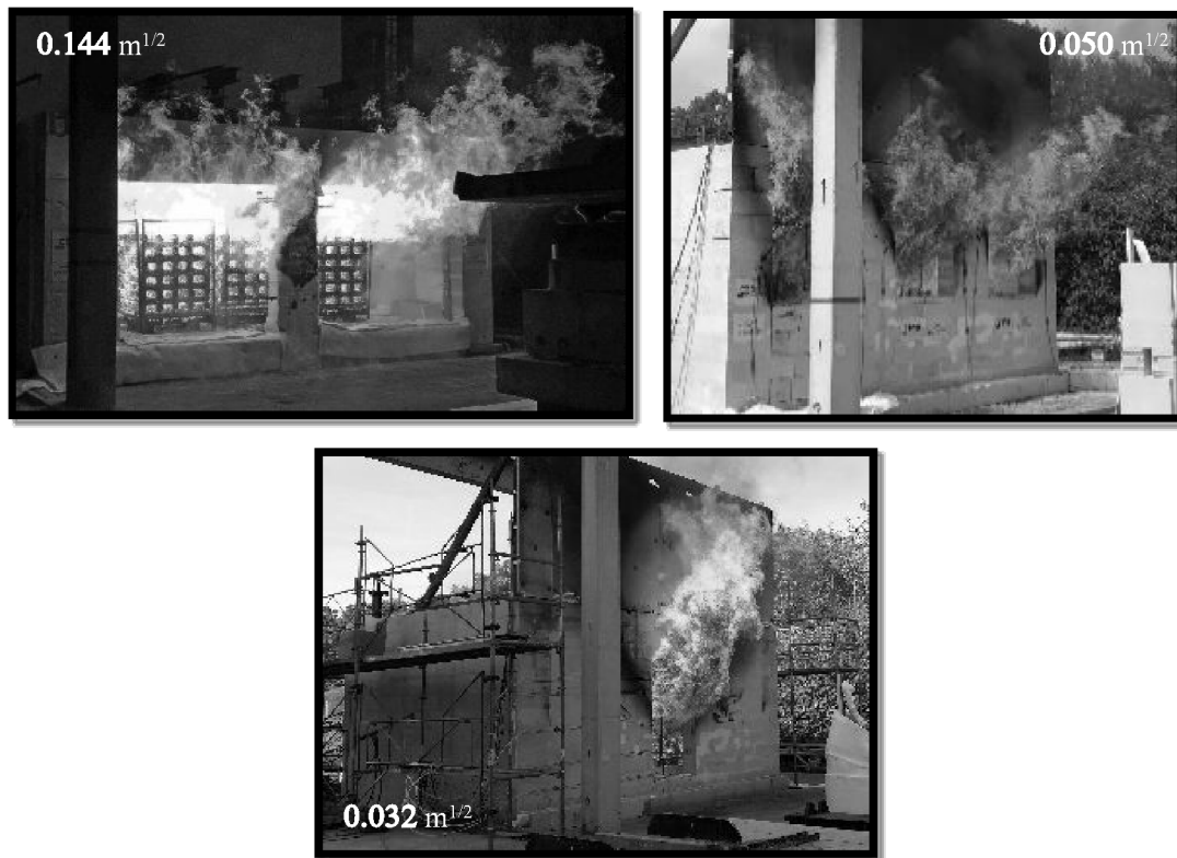
Figure 2. CLT slabs tested with three different opening configurations; opening factors were 0.144, 0.050, and 0.032 m 1/2 .
