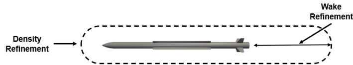
Fig. 6 Density and wake refinement regions recorded in the key mesh metrics spreadsheet, including size and cell edge length of both the density and wake refinement areas.
