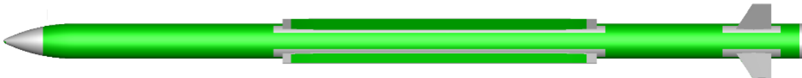
Fig. 15 Partition of the surface mesh into area with rectangular elements (green) and triangular elements (grey).
