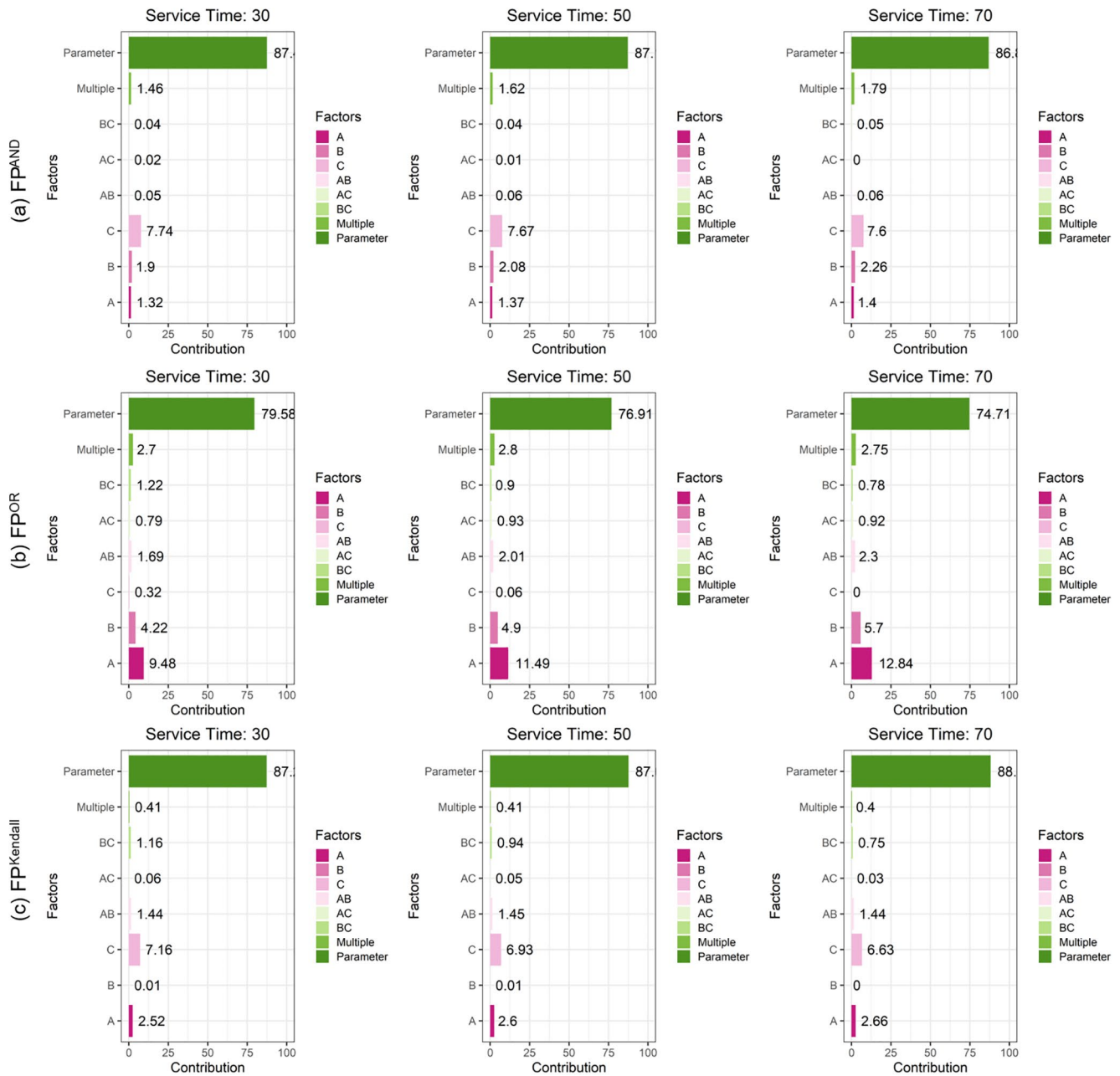
Figure 9. The main effects of uncertain factors and their interactions on the predictive uncertainties for FPs obtained by the FMBC method at Washington.
